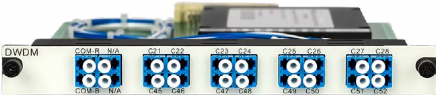
DWDM (Dense Wavelength Division Multiplexing) Placas modulares Mux/Demux de 4, 8, 16 canais.
